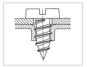
Fig. 4: Tapping hole drawn through (thin plates)
