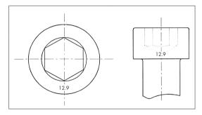
Fig. H: Example for the marking of socket head cap screws
