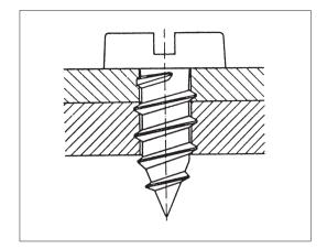
Fig. 1: Simple screwed joint (two tapping holes)
