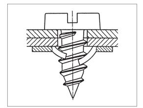
Fig. 6: Screwed joint with tightening nut
