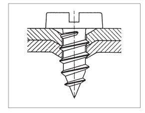
Fig. 3: Tapping hole, widened (thin plates)
