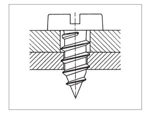
Fig. 2: Simple screwed joint with through hole
