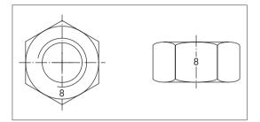
Fig. I: Example of marking with the code number of the strength class
