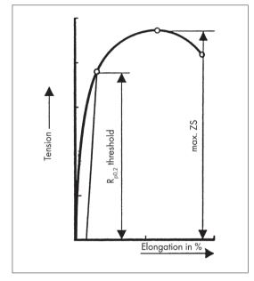
Stress-strain diagram of a screw with strength class 10.9 (qualitative)
